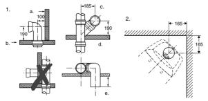
1. S+Q a. Finished wall b. Finished floor c. Drainage pipe dim 110/45 d. WC-connection e. Cut to suitable length
